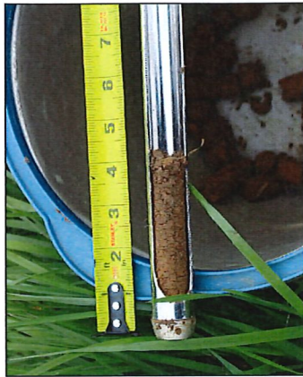
Figure 2. A soil probe should always be used to collect soil samples. Sampling depth for pastures and hayfields should be 4 inches.
